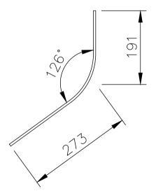
CEMBRIT LIMITED CEMSIX APRON FLASHING PIECE LENGTH: 1060mm NET COVER: 1016mm AVAILABLE IN LEFT AND RIGHT HANDED VERSIONS Drg. No.420
